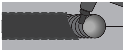
PARTIALLY CHIPPED AWAY TO SHOW WELD
